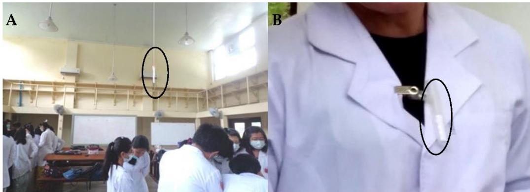
Figure 2. Diffusive air samplers: (A) air samplers placed in dissection room for indoor FA concentration; and (B) attached to the breathing zone for personal FA exposure.
